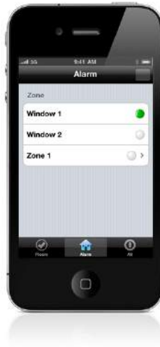
Fig 6.22: Example of usage of the Status element to visualize state of an alarm zone
