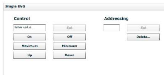
Fig 13.3: Panel to manage a single ballast
