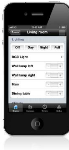
Fig 6.6: Exemplary section for lighting control.
